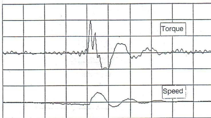
Figure 2: Measured performance of the simulated induction motor under the same, specified conditions
