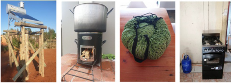
Figure 6: The four technologies identified for evaluation in the wood-using households, from left to right: solar water heater on a wooden stand, rocket stove, Wonderbag and LPG stove
