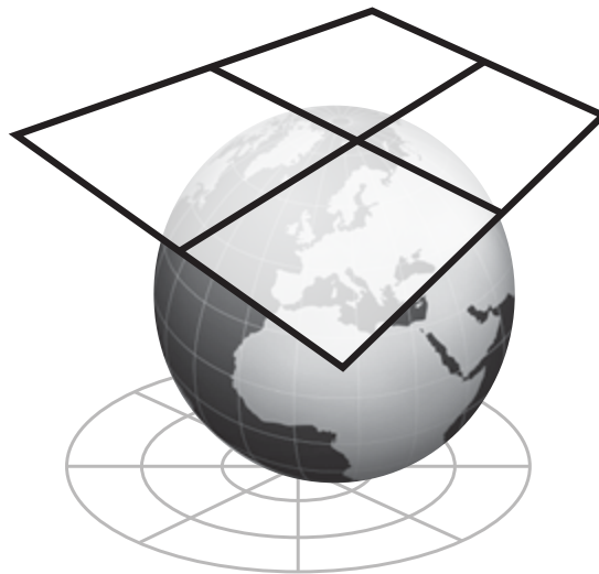
Illustration of how a two-dimensional map is derived from a three-dimensional globe
